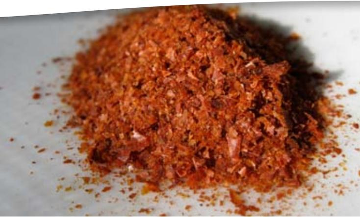
The main objective of the project is the production of a pilot plant for the extraction of the cutin from industrial tomato by-products. The cutin, a component of the tomato skins, is the starting material that will be used for the production of a bio-lacquer for the protection of metal food packaging.
